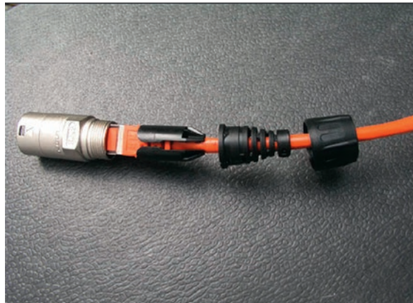
Fig. 11 The Ethernet Cable will be inserted into the plug like this. The parts are pressed into the metal mantle by screwing the black plastic nut (rightmost part) onto the mantle .
