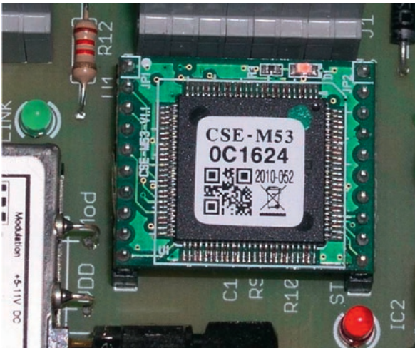
Fig. 8 Ethernet-Interface module CSE-M53 in the transmitter. The last six digits of the MACaddress) are printed on the label (0C1624 in this example).
