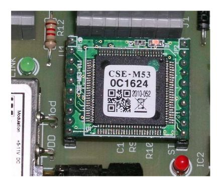
Fig.8 Ethernet-Interface module CSE-M53 in the transmitter. The last six digits of the MAC-address) are printed on the label (0C1624 in this example). The MAC address identifies the Ethernet module within the network. The MAC adress is neither to be confused with the device number on the DIP-switch nor with the IP-address.
