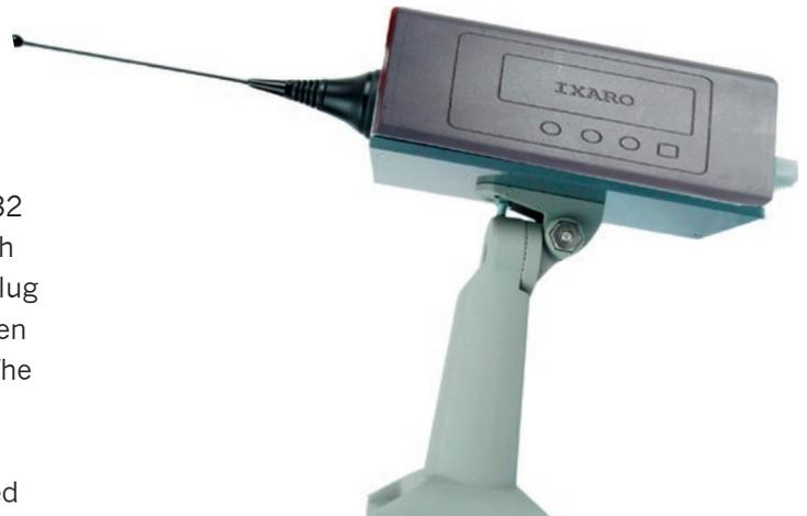
The IXARO Standard transmitter may be used also without a computer to send predefined messages triggered by one of two switches. The connection of the switches is also made at the 9 pold D-Socket. When one of the switches is closed the message assigned to that input will be sent. Assignment of the messages is explained in the description of the IXARO software. The following schematic shows how to connect the switches:
