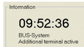
When the power supply to the terminal is interrupted, the message disappears. If the wires A and B from the terminal have been swapped by mistake an error message appears and the terminal will be deactivated:
