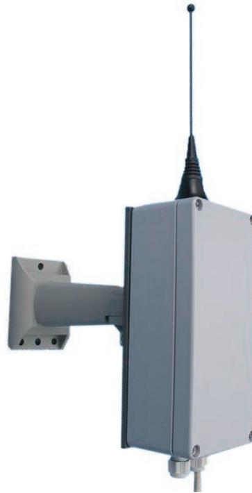
Up to eight transmitters of the IXAROBUS-series may be operated on one cable (RS422-BUS). The transmitters are wired parallel. This cable contains also the power supply wires. Thus even bigger areas can be supplied with the wireless signal. The cable may have a length up to 1.500 meters.
